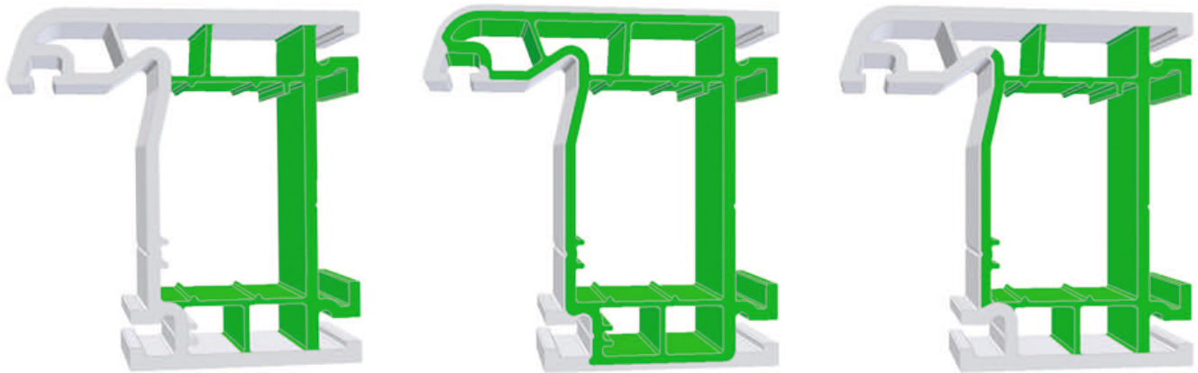
Fig 1. Co-extrusion using core, layer and combination technologies (from left to right) (picture: Greiner Extrusion)
