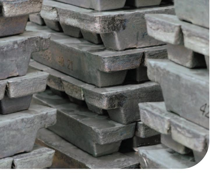
The starting material for all Baerlocher lead products is high purity lead metal.
